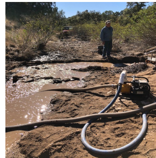
Chris Lespron builds a temporary dam to supply water for his high-banker.
